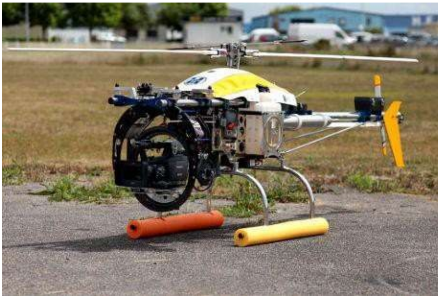
Fig 2.8)Single Rotor drone
